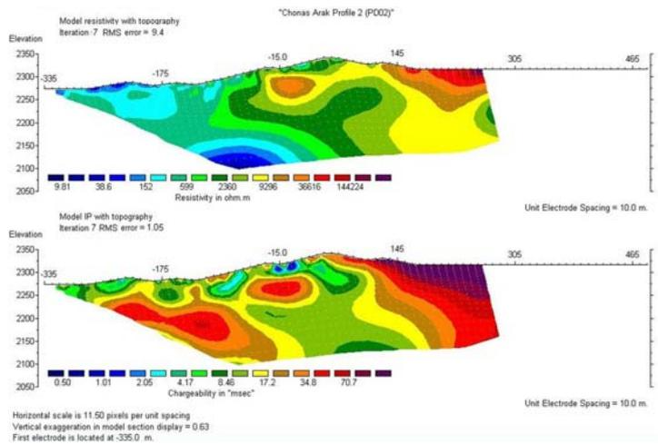
Figure-3. IP and Resistivity models of pole-dipole profile with Topographic correction and without changing Inversion parameters.
