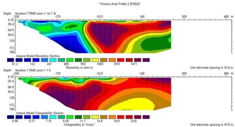
Figure-2. IP and Resistivity models of pole-dipole profile without Topographic correction and with changing Inversion parameters.
