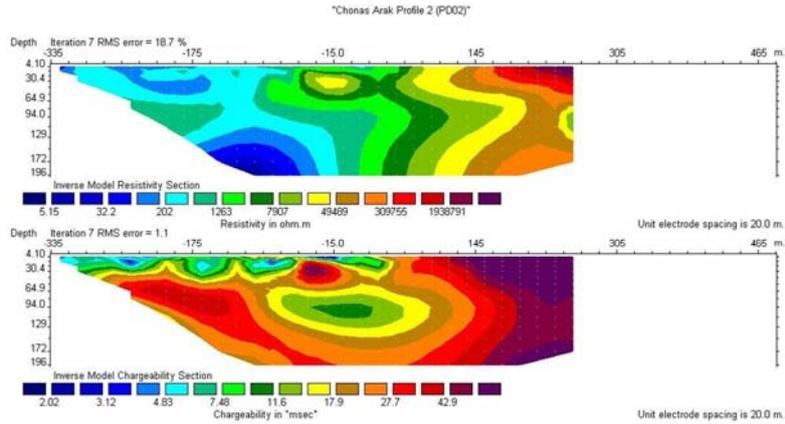
Figure-1. IP and Resistivity models of pole-dipole profile without Topographic correction and changing Inversion parameters.
