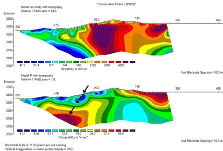
**Figure-4.** IP and Resistivity models of pole-dipole profile with Topographic correction and changing Inversion parameters. Bold arrows show the best site for exploration drilling.
