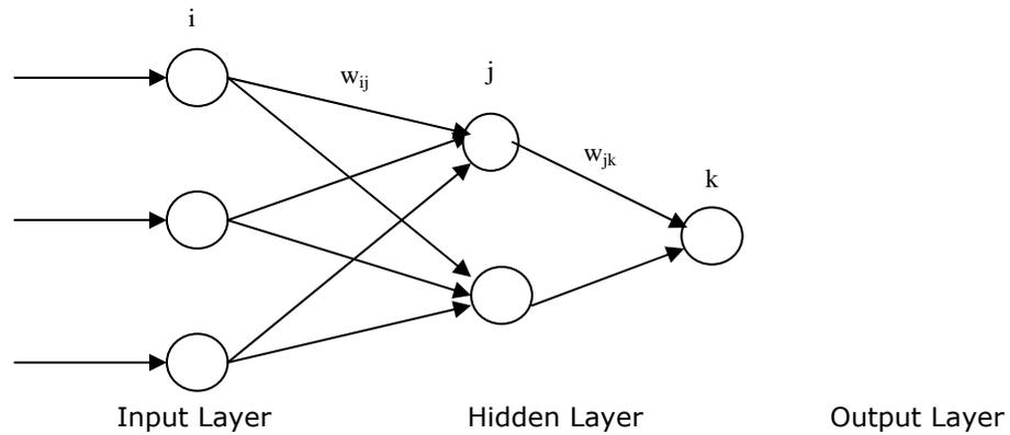
**Fig. 1** A typical three-layer feed forward ANN
