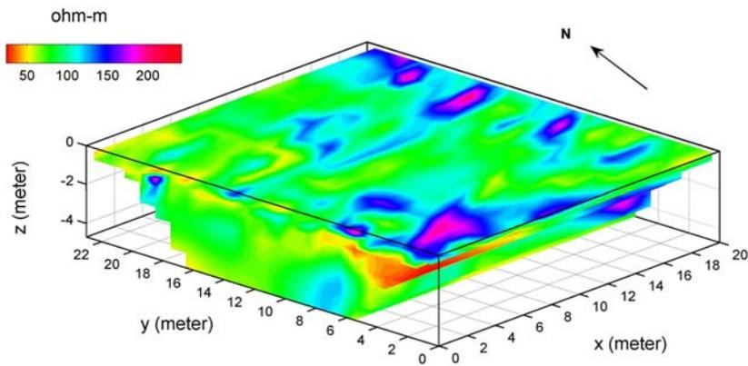
**Figure-3.** 3D resistivity imaging of the Area2 obtained from the inversion of 2D profiles
