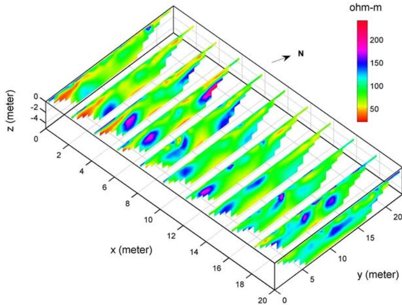
**Figure-2.** The 2D model resistivity sections of the 11 pole-dipole profiles
