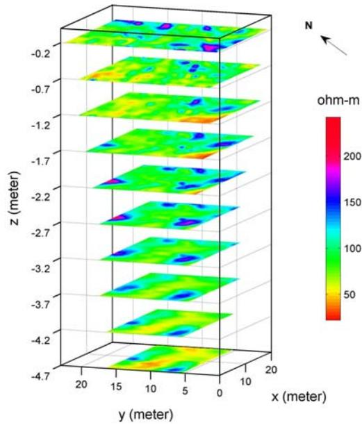
**Figure-4.** Horizontal depth slices of the resistivity distribution
